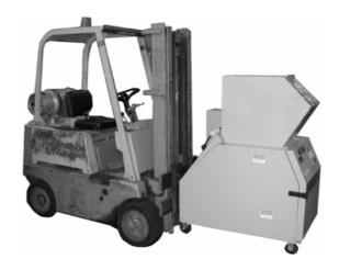
Figure: Lifting the granulator
